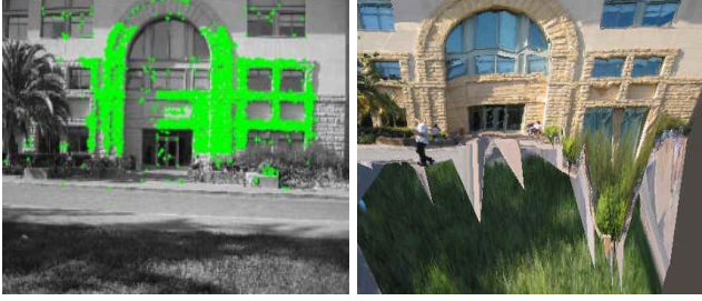
Figure 6. An image showing a few matches, and the resulting 3-d model without estimating the variables y for confidence in the 3-d matching. The noisy 3-d matches reduce the quality of the model. (Note the cones erroneously projecting out from the wall.)
