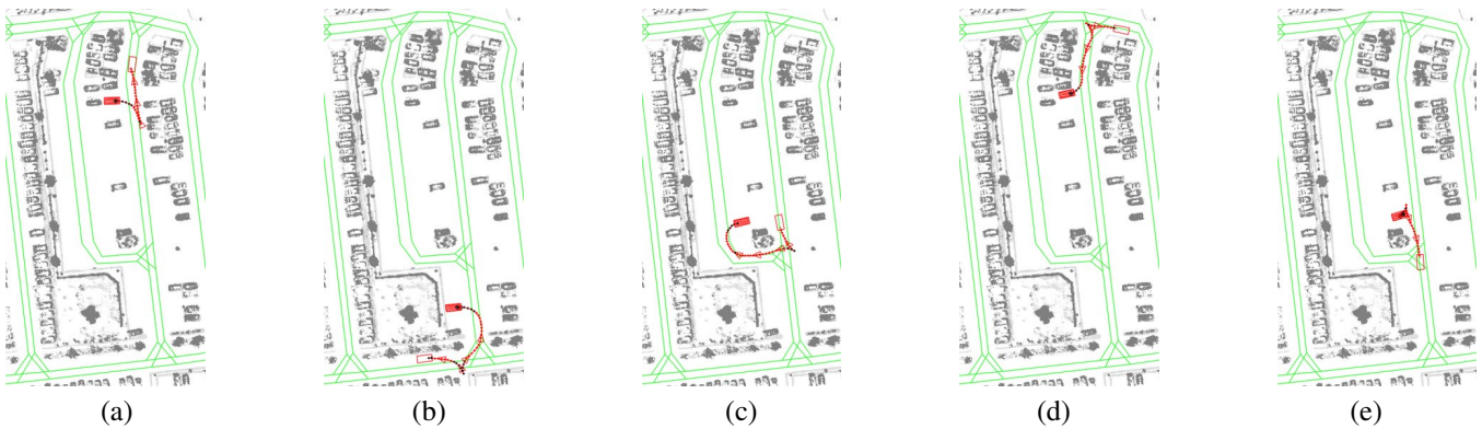
Fig. 9. “Backward” parking lot navigation driving: trajectories found by learning on four demonstrations, and testing on the fifth. (See text for details.)
