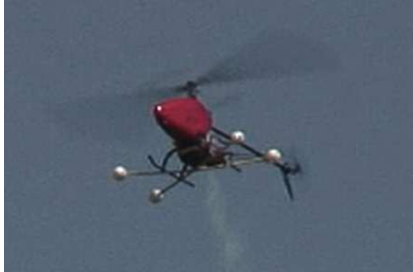
Fig. 1. Instrumented XCell Tempest during autonomous autorotation.
