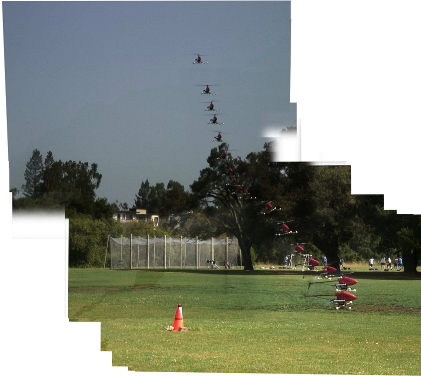
Fig. 5. Mosaic of one of our autonomous autorotation flights as viewed from in front of the helicopter. (Sampled at 4Hz.)
