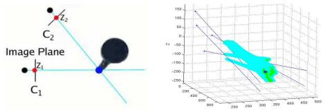
Figure 4: (a) Diagram illustrating rays from two images  $C_1$  and  $C_2$  intersecting at a grasping point (shown in dark blue). (b) Actual plot in 3-d showing multiple rays from 4 images intersecting at the grasping point. All grid-cells with at least one ray passing nearby are colored using a light blue-green-dark blue colormap, where dark blue represents those grid-cells which have many rays passing near them. (Best viewed in color.)
