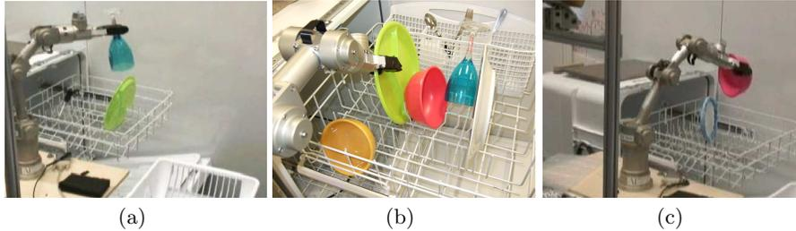
**Fig. 6.** Dishwasher experiments (Section 6.2): Our robotic arm unloads items from a dishwasher.
