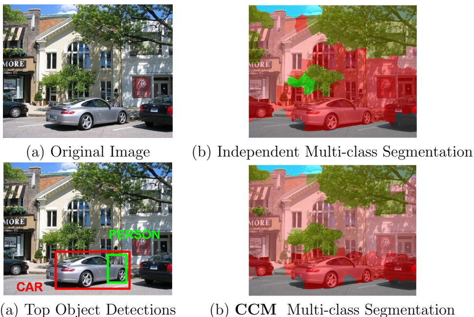
Figure 4.15: Example image from the DS1 dataset (a), where the independent multi-class segmentation (b) puts too much ‘foreground’ in the middle of the image (where the building is). Once it sees the detections (c), however, the final segmentation correctly identifies the building and the trees above the car.
