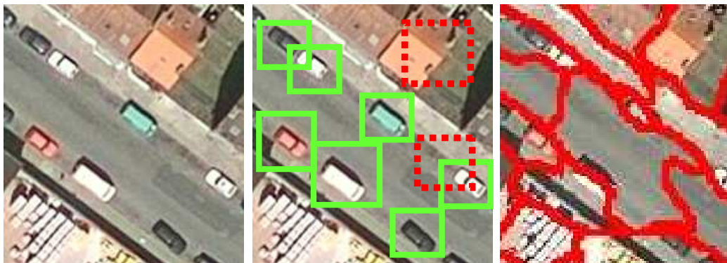
Figure 5.1: (Left) An aerial photograph. (Center) Detected cars in the image (solid green = true detections, dashed red = false detections). (Right) Finding “stuff” such as buildings, by classifying regions, shown delineated by red boundaries.
