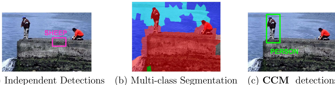
Figure 4.14: Example image from the DS1 dataset, where the original top detection (a) is a sheep, but after considering the segmentation (b), resulting a correct final detection (c) of the person.
