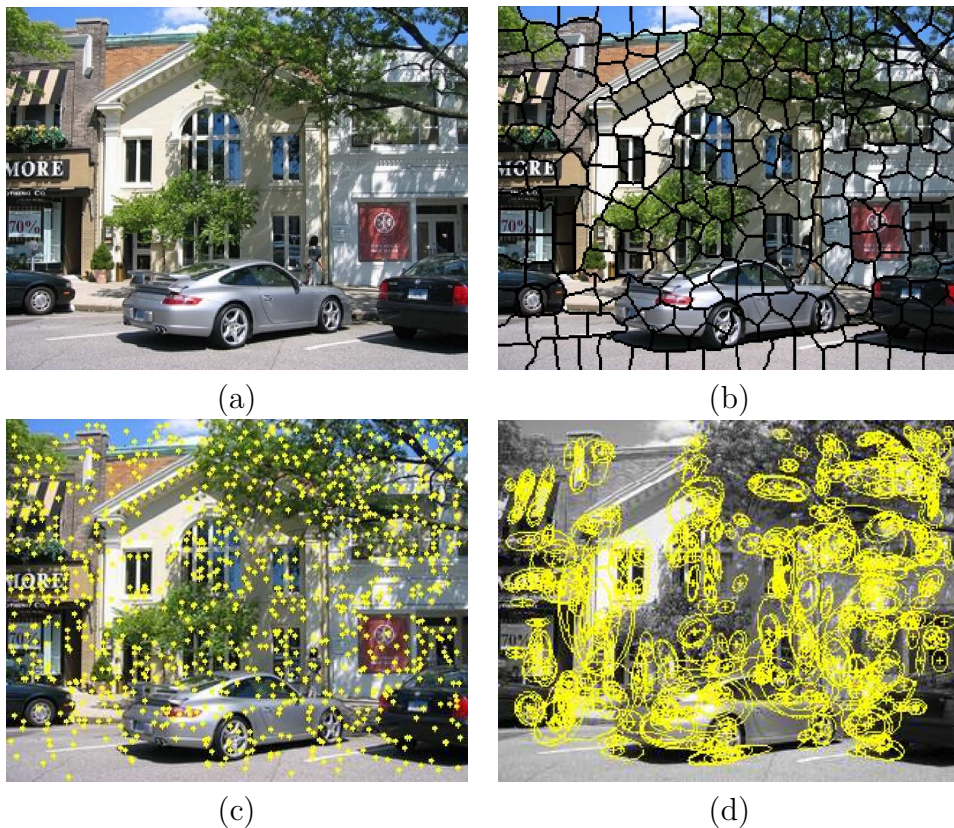
Figure 3.2: (a) An image of a street scene. (b) An oversegmentation of the image into coherent regions that are often called “superpixels.” (c) A sparse segmentation of the image into interest points that are selected using the SIFT keypoint detector. (d) keypoints extracted by the Harris-Affine keypoint detector of Mikolajczyk and Schmid [91]. It is often assumed that these keypoints will represent the important locations in the image, such as objects and boundaries between substructures.
