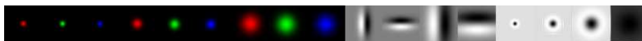
Figure 2.3: Illustration of texton filters. Note that the filters operate in CIELab color space (RGB shown for illustrative purposes only).
