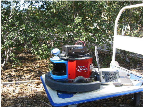
Figure 2. Rig for collecting correlated laser range scans and real camera images.
