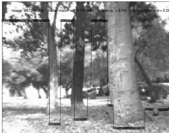
Figure 1. Laser range scans overlaid on the image. Laser scans give one range estimate per degree.
