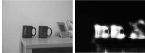
Figure 4: Learned interest. The righthand panel shows the probability of interest for each pixel in the peripheral image (left).
