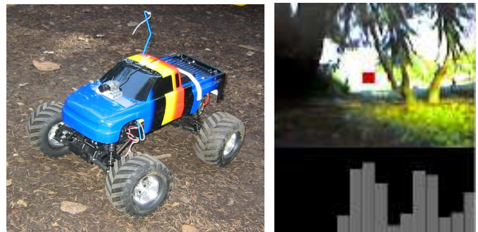
Figure 11: (a) The remote-controlled car driven autonomously in various cluttered unconstrained environments, using our algorithm. (b) A view from the car, with the chosen steering direction indicated by the red square; the estimated distances to obstacles in the different directions are shown by the bar graph below the image.
