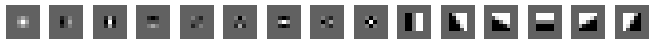
Figure 2: The convolutional filters used for texture energies and gradients. The first nine are 3x3 Laws’ masks. The last six are the oriented edge detectors spaced at 30^\circ intervals. The nine Laws’ masks are used to perform local averaging, edge detection and spot detection.
