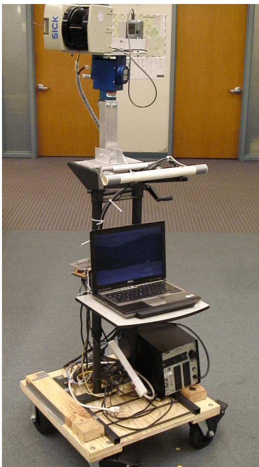
Figure 7: The 3-d scanner used for collecting images and the corresponding depthmaps.
