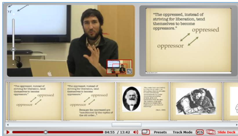
Screenshot 5: ClassX system by Bernd Girod. System allows pan/zoom during playback, and features slide synchronization. ( http://classx.stanford.edu/ )
