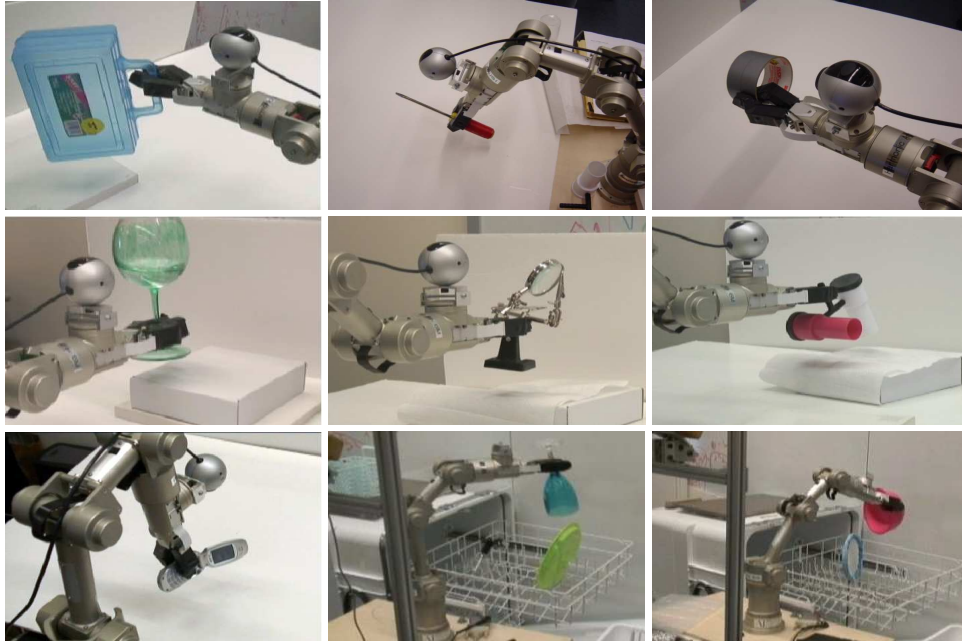
Figure 6: The robotic arm picking up various objects: box, screwdriver, duct-tape, wine glass, a solder tool holder, powerhorn, cellphone, and martini glass and cereal bowl from dishwasher.
