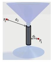
Figure 4: An illustration showing the grasp labels. The labeled grasp for a martini glass is on its neck (shown by a black cylinder). For two predicted grasping points  $P_1$  and  $P_2$ , the error would be the 3-d distance from the grasping region, i.e.,  $d_1$  and  $d_2$  respectively.
