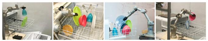
Figure 14: Dishwasher experiments (Section 6.3): Our robotic arm unloads items from a dishwasher.
