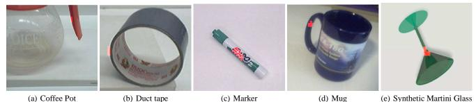
(a) Coffee Pot (b) Duct tape (c) Marker (d) Mug (e) Synthetic Martini Glass Figure 7: Grasping point classification. The red points in each image show the locations most likely to be a grasping point, as predicted by our logistic regression model. (Best viewed in color.)
