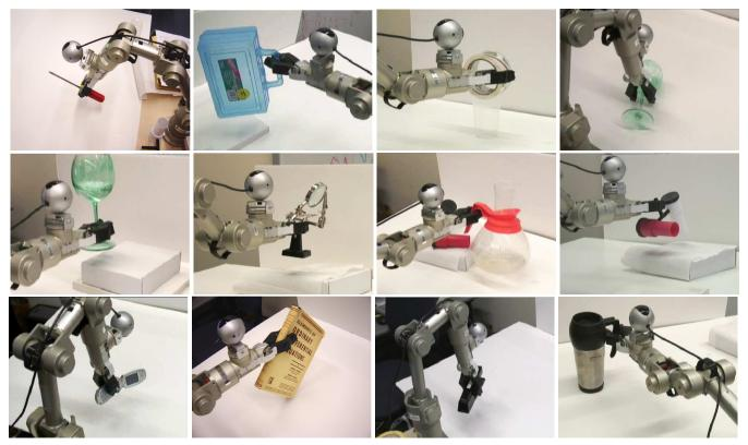
Figure 11: The robotic arm picking up various objects: screwdriver, box, tape-roll, wine glass, a solder tool holder, coffee pot, powerhorn, cellphone, book, stapler and coffee mug. (See Section 6.2.)
