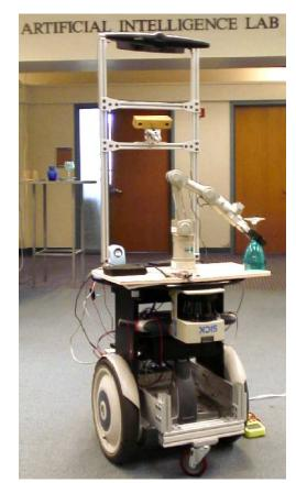
Figure 9: STAIR 1 platform. This robot is equipped with a 5-dof arm and a parallel plate gripper.
