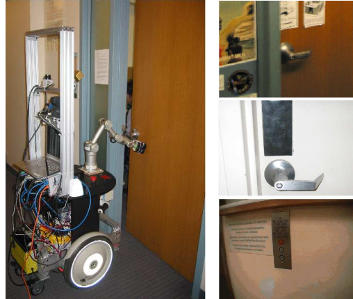
Fig. 1. Variety of manipulation tasks required for a robot to navigate in the environment.
