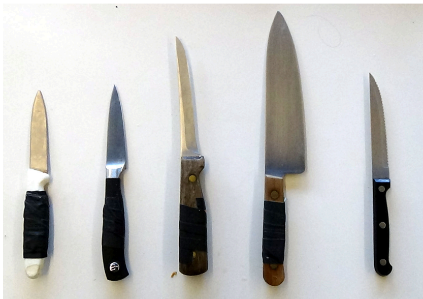
Figure 3.10: Different tools: Different knives used to test my algorithm. From left to right, the paring knife used to collect data and train the algorithm, a shorter, sharper paring knife, a long kitchen knife, a wedge-shaped chef's knife, and a serrated steak knife. In all cases except the serrated knife, my algorithm, trained only with the paring knife on the left, was able to maintain comparable cutting rates.
