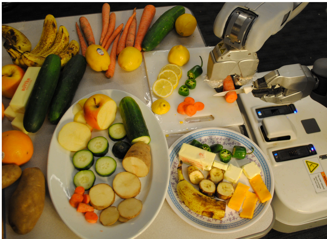
Figure 3.1: Cutting food: My PR2 robot uses my algorithms to perform complex, precise food-cutting operations. Given the large variety of material properties, it is challenging to design appropriate controllers.
