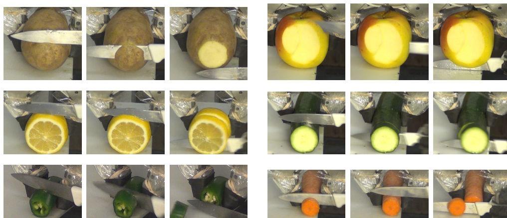
Figure 3.9: Cutting food: Time-series of my PR2 robot using my DeepMPC controller to cut several of the food items in my dataset. My algorithm is able to adapt its strategy for different materials. Note in particular that it picks up the knife slightly, then chops back down when cutting the carrot, and uses more “sawing” motion on tougher materials. Video of these experiments is available at http://deepmpc.cs.cornell.edu
