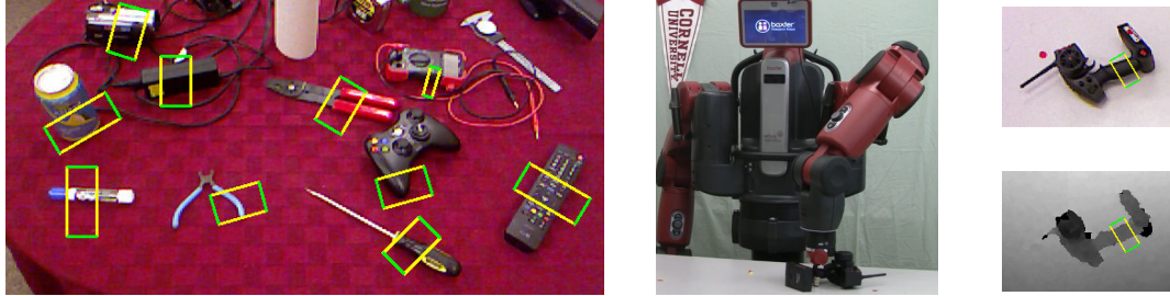
Figure 2.1: Detecting robotic grasps: Left: A cluttered lab scene labeled with rectangles corresponding to robotic grasps for objects in the scene. Green lines correspond to robotic gripper plates. I use a two-stage system based on deep learning to learn features and perform detection for robotic grasping. Center: A Baxter robot “Yogi” successfully executing a grasp detected by my algorithm. Right: The grasp detected for this case, in the RGB (top) and depth (bottom) images obtained from Kinect.
