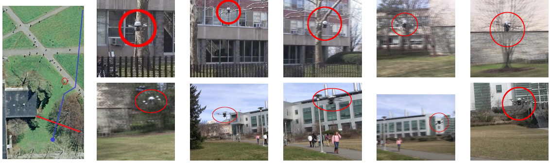
Figure 4.8: Avoiding obstacles in series: My aerial robot avoiding a fence and a pole in sequence. Left: Overhead map of area, red indicates obstacles avoided, blue robot path. Robot started at the blue dot, behind and below the level of the fence, moved upwards to a safe altitude, and proceeded over the fence and through the clear area. It then stopped at the pole, detected it as an obstacle, moved diagonally to the right to avoid it, and then forwards again through the following clear area.
