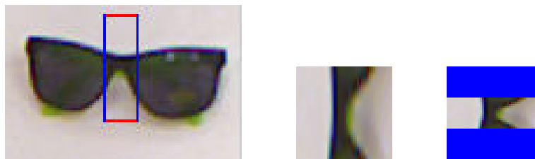
Figure 2.4: Preserving aspect ratio: Left: a pair of sunglasses with a potential grasping rectangle. Red edges indicate gripper plates. Center: image taken from the rectangle and rescaled to fit a square aspect ratio. Right: same image, padded and centered in the receptive field. Blue areas indicate masked-out padding. When rescaled, the rectangle incorrectly appears graspable. Preserving aspect ratio and padding allows the rectangle to correctly appear non-graspable.
