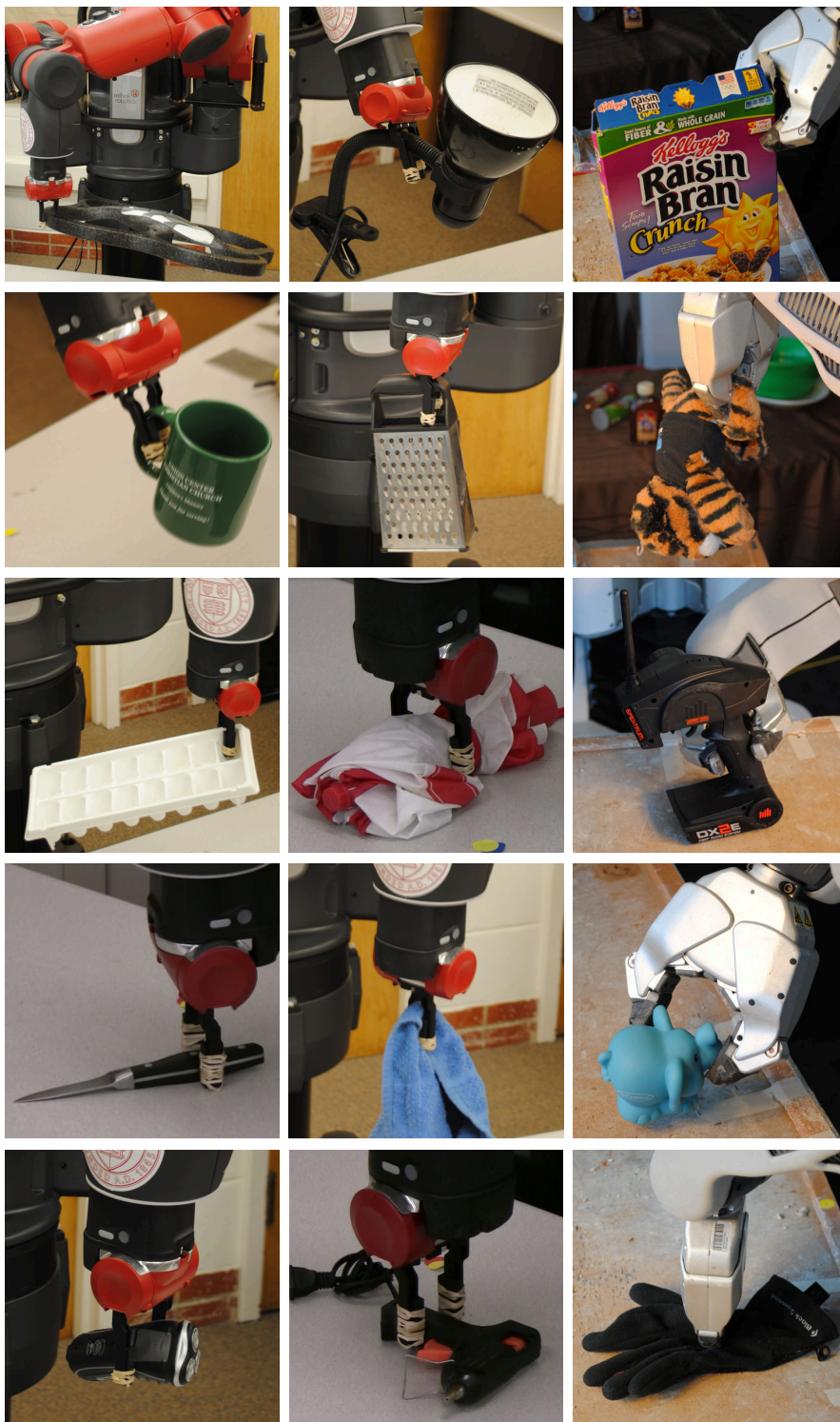
Figure 2.14: Robots executing grasps: My robots grasping several objects from the experimental dataset. Top row: Baxter grasping a quad-rotor casing, coffee mug, ice cube tray, knife, and electric shaver. Middle row: Baxter grasping a desk lamp, cheese grater, umbrella, cloth towel, and hot glue gun. Bottom row: PR2 grasping a plush cat, RC car controller, cereal box, toy elephant, and glove.
