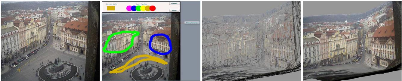
**Figure 1:** (a) An original image. (b) Interactive tool: user draws over the image in 5-10 seconds. (c) The 3-d model predicted by the algorithm. (d) A screenshot of the textured 3-d model. (Also see attached video.)
