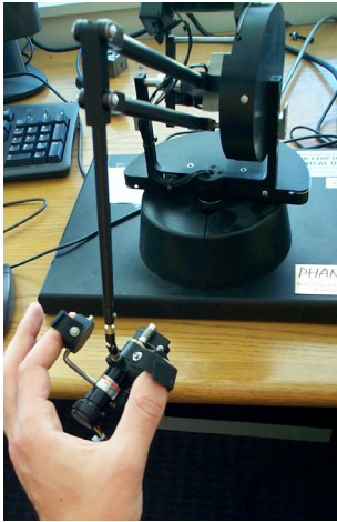
Figure 2. A device with four motors and four sensors allowing users to grasp and manipulate virtual objects
