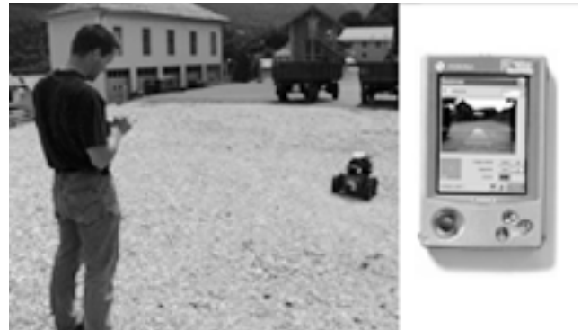
Figure 4. PdaDriver is a PDA-based interface for remote driving.
