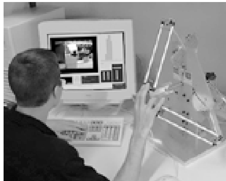
Figure 3. HapticDriver provides force feedback for precision driving tasks.
