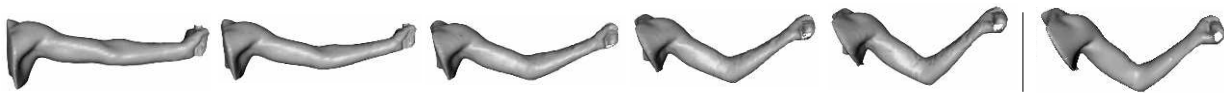
Figure 8: Several frames from a motion animation generated by interpolating two scans of an arm (far left and far right), which were automatically registered using the Correlated Correspondence algorithm. The animation was produced by linear interpolation in link transformation space.
