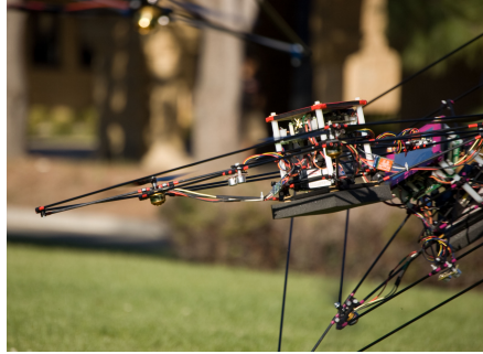
Figure 14: A mid-air collision between two out of three remote-piloted quadrotor helicopters operating in close proximity. The proposed algorithm would assume control when required to prevent imminent collisions.
