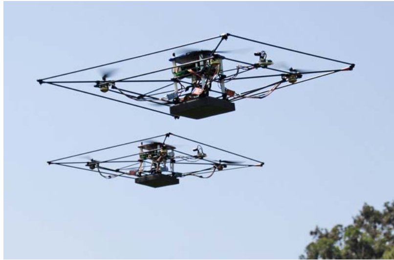
Figure 1.1: Two quadrotor helicopters from the Stanford Testbed of Autonomous Rotorcraft for Multi-Agent Control (STARMAC) in autonomous hover control at GPS waypoints.
