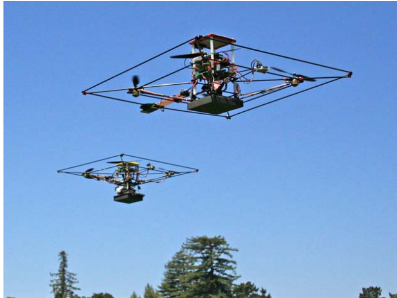
Figure 5.22: Two STARMAC quadrotor helicopters flying with avalanche rescue beacon transceivers.
