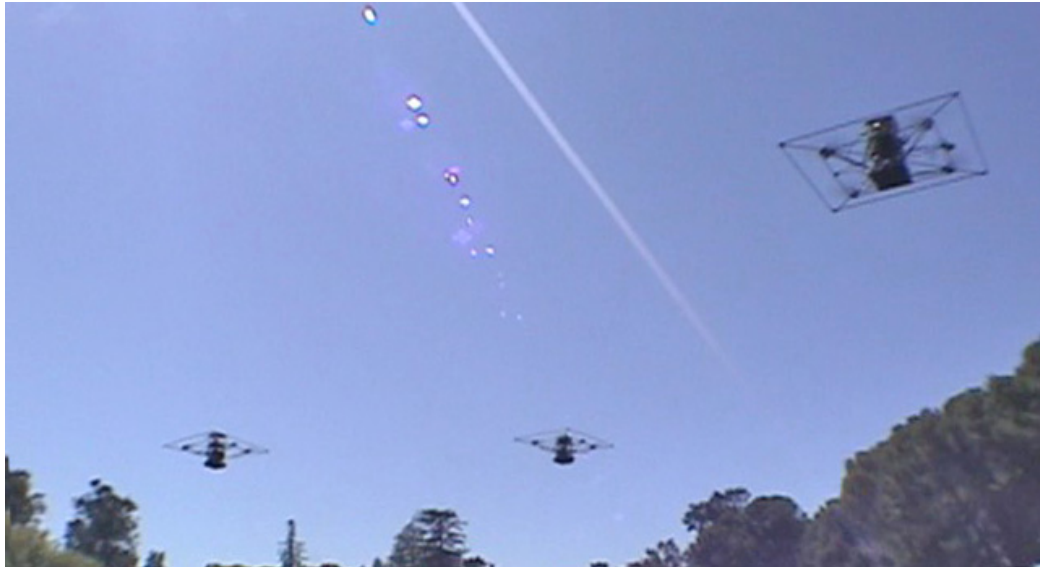
Figure 2.15: Three STARMAC quadrotor helicopters performing position control at GPS waypoints.
