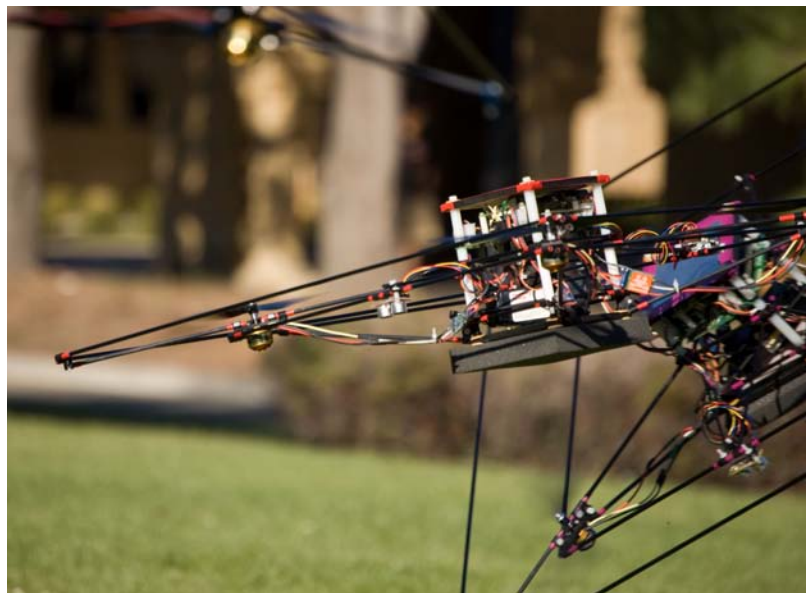
Figure 4.1: A mid-air collision between two out of three remote-piloted quadrotor helicopters operating in close proximity. The proposed algorithm would assume control when required to prevent imminent collisions.
