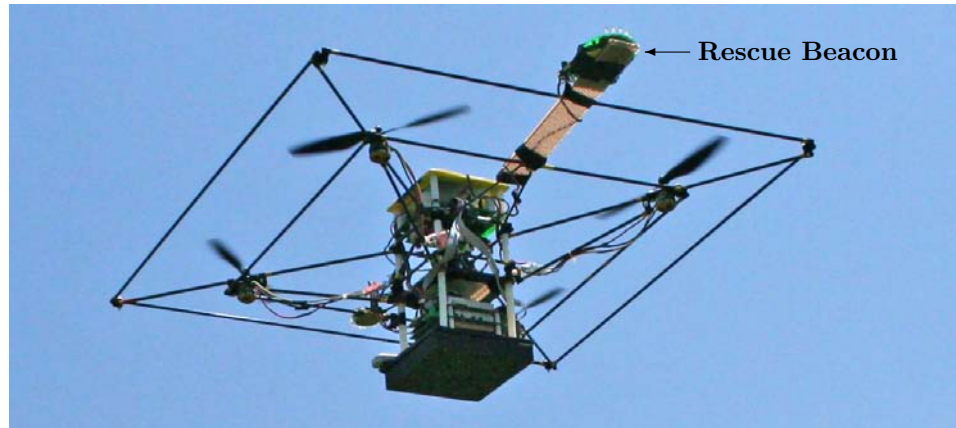
Figure 5.20: A STARMAC quadrotor helicopter with a avalanche rescue beacon transceiver.
