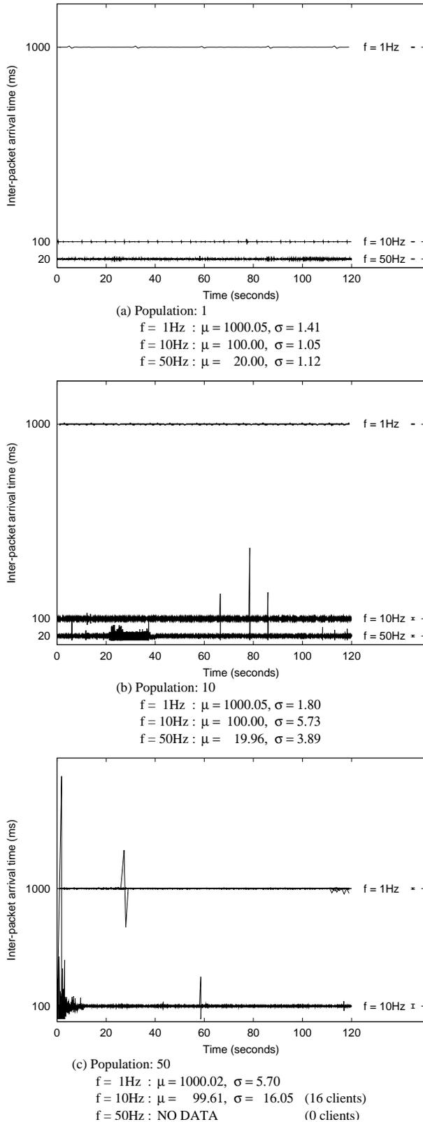
**Figure 3:** Inter-packet arrival times measured while serving large amounts of sensor data across wireless Ethernet to different client populations.
