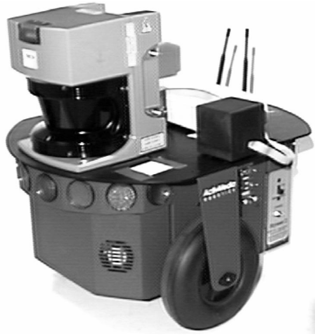
Fig. 1. Typical Pioneer 2-DX robot. Visible in this image are the two drive wheels, front sonar ring, compass (small cube), Ethernet modem (antennae protruding vertically) and laser range finder (looks like a coffee maker). At the rear of the robot is another ring of sonars.
