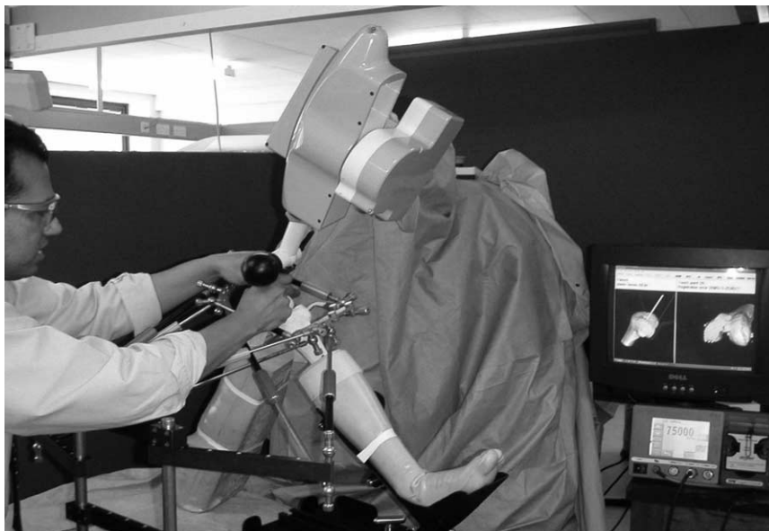
Fig. 4. Acrobot Active Constraint Knee Arthroplasty System. (Courtesy of the Acrobot Company Limited, London, England.)
