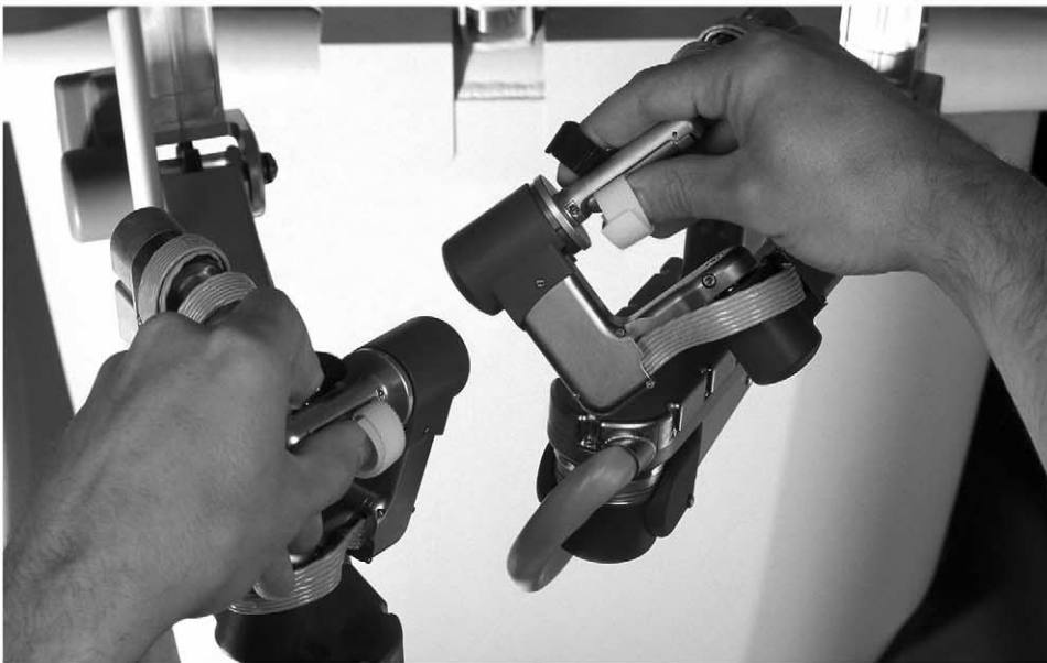
Fig. 7. The da Vinci EndoWrist ( top ) and console masters ( bottom ). The wristed slave instruments exactly track the surgeon's master controllers. (Courtesy of Intuitive Surgical, Inc., Sunnyvale, CA.)
