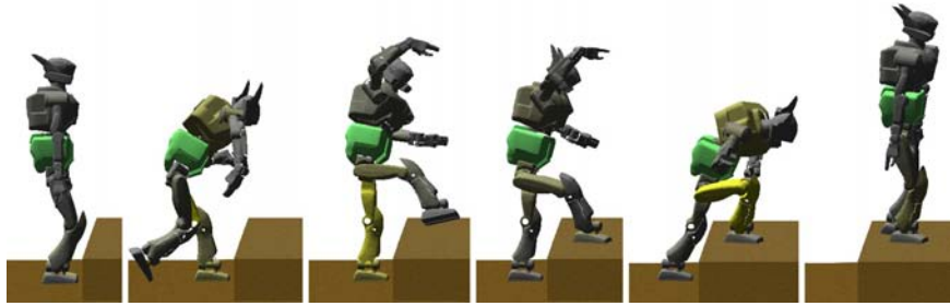
Fig. 4. Stair step planned entirely from scratch.
