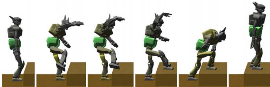
Fig. 5. Primitives guide path planning, reducing unnecessary leg motions.
