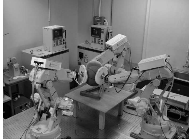
Fig. 2. HKUST 3-fingered hand manipulating a spherical object.
