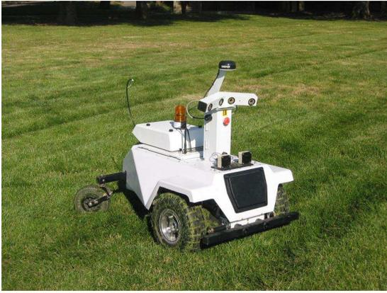
Fig. 1. Ground rover platform instrumented with inexpensive IMU and GPS. This robot is commercially provided to contractors in the DARPA LAGR program.
