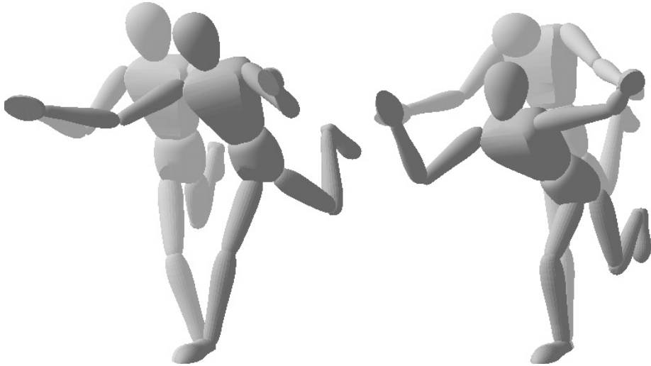
Fig. 1. Redundancy: These superimposed images display the redundancy property for a given task. The robot can take multiple configurations while maintaining fixed locations for its hands.
