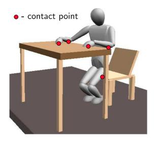
The spacial selection matrices will be defined by the contact normal directions of all the operational points :  $\Omega_f(n_1, n_2, \ldots, n_l)$  and  $\Omega_m(n_1, n_2, \ldots, n_l)$
