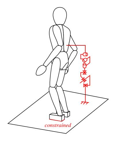
$$A(q)\ddot{q} + b(q,\dot{q}) + g(q) + J_c^T (f_c) = \Gamma$$
