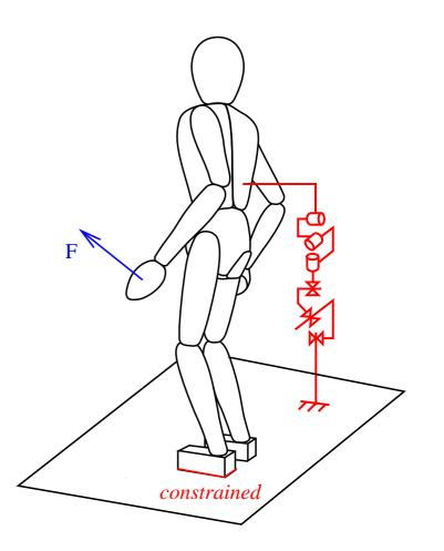
The relation between joint torque and force
