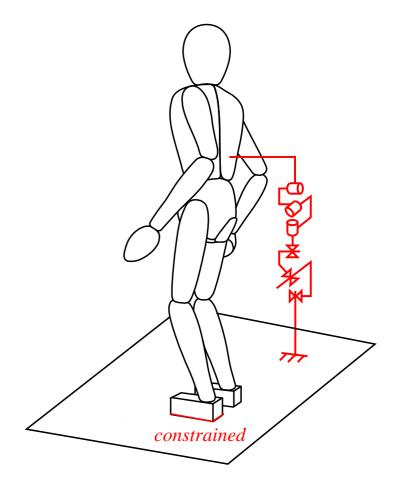
$$A(q)\ddot{q} + b(q,\dot{q}) + g(q) + J_c^T (f_c) = \Gamma$$
