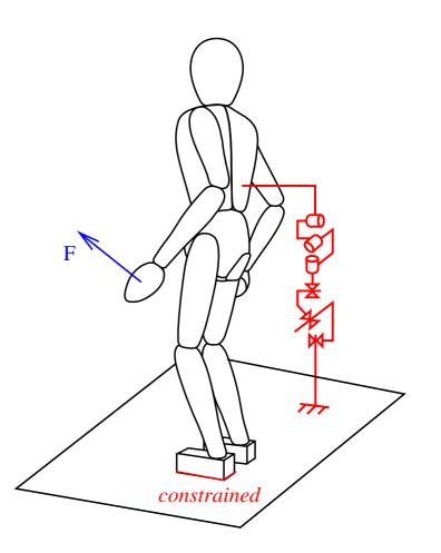
The relation between joint torque and force
