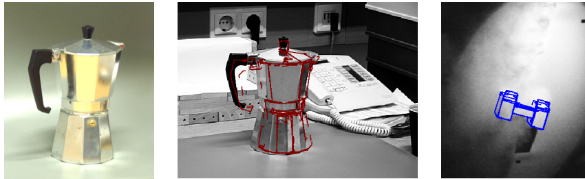
Fig. 4. Real training image (left) and recognition result (middle) for a highly specular object. Detected barbell (right) under extensive occlusion by fog.
