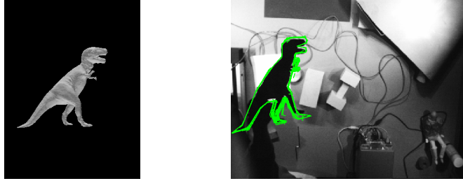
Fig. 1. One of the generated training images (left) and the recognition result (right) for a free-form object. It was sufficient for this object to learn and represent the silhouette.
