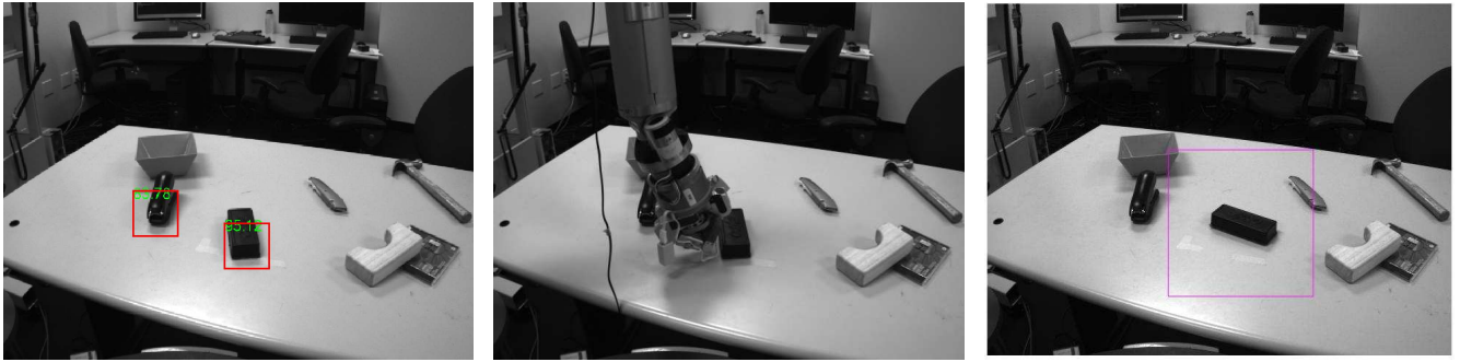
(a) First view of the scene. Which one of the objects shown in red boxes is a stapler? (b) The robot perform actions to rotate them in order to get better views. (c) View after first action (using our method).
