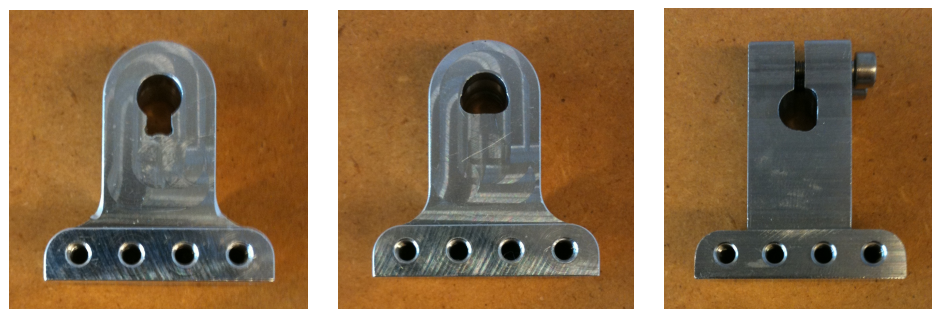
(a) Connector version I (b) Connector version II (c) Connector version III
