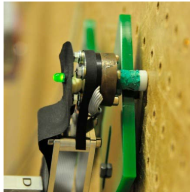
(b) The shaft of the force sensor is the finger.
