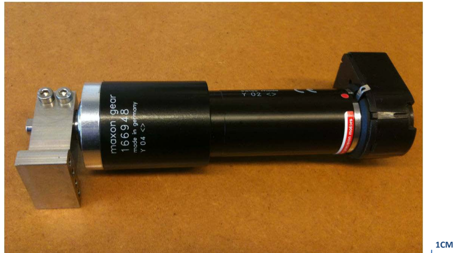
Figure 2.7: Actuator set for each joint. From left to right: connector, gearhead, motor, and encoder.
