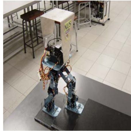
Fig. 14. Experiment of RoboSapien walking on stairs.
