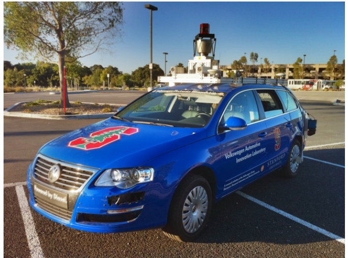
Fig. 1: Junior, the autonomous driving platform.
