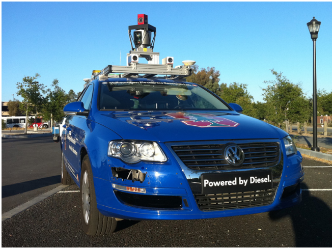
Fig. 2: Junior, the autonomous vehicle research platform. In this work, we use a Velodyne dense LIDAR sensor and an Applanix inertial measurement unit to track objects while moving.
