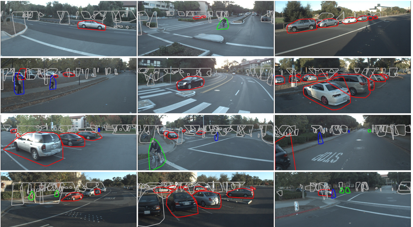
Fig. 8: Track classifications in LIDAR data projected into aligned camera data for visualization. Best viewed in color. Cars are outlined in red, pedestrians in blue, bicyclists in green, and background in gray. Objects without outlines were not tracked. Tracking and segmentation errors (beyond the scope of this paper) are the major cause of failures. A video of these results can be seen at [20].
