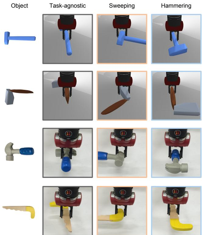
Figure 7: **Qualitative results.** Column 1 shows RGB images of the tool objects. Column 2 shows example task-agnostic grasps. And Columns 3 and 4 show task-oriented grasps chosen by our model for the sweeping and hammering tasks. Our model favors wide flat surfaces for sweeping and long moment arms for hammering.
