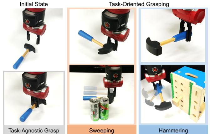
Figure 1: The same object can be grasped by the robot in different ways from the initial state on the table. A task-agnostic grasp can lift up the hammer but it might not be suitable for specific manipulation tasks such as sweeping or hammering. We aim to directly optimize for task success in each episode, by jointly choosing a task-oriented grasp and the subsequent manipulation actions.
