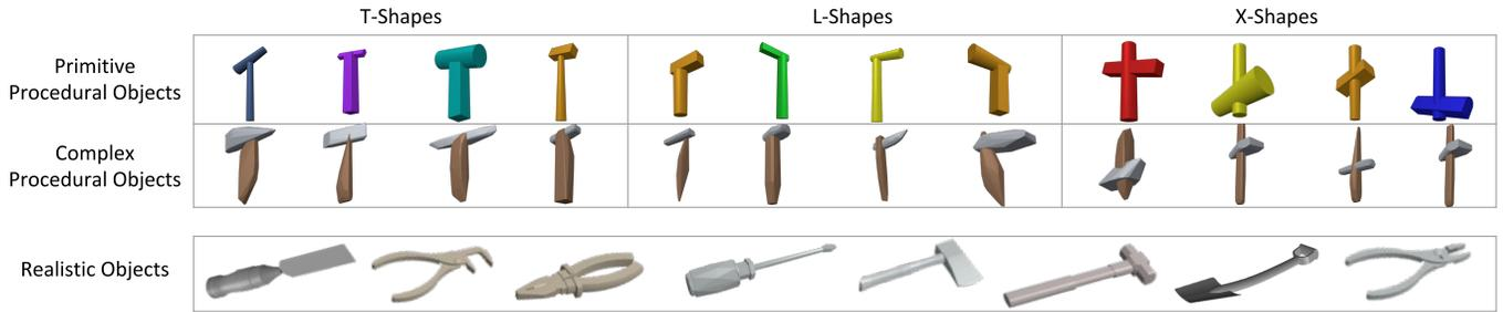
Figure 4: **Example of objects in simulation.** The first two rows show the procedurally generated objects based on shape primitives as well as complex meshes. These objects are generated using three predefined composing rules to result in T-shapes, L-shapes, and X-shapes. The last row shows the realistic shapes from existing 3D model datasets.
