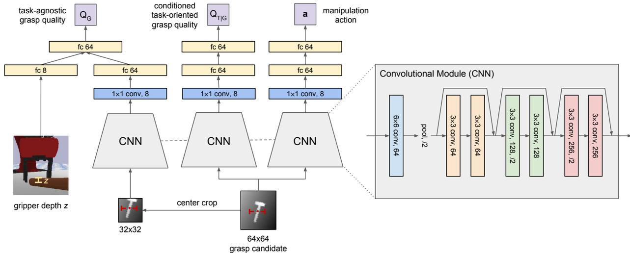
Figure 3: **Task-Oriented Grasping Network (TOG-Net)**. The inputs to the network are two depth image crops and the sampled gripper depth  $z$ . The network predicts task-agnostic grasp quality, conditioned task-oriented grasp quality, and manipulation actions. The CNN modules share parameters as denoted by the dashed lines. Residual network layers and batch normalization are used in the CNN modules.
