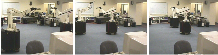
Figure 3. Execution of a plan using the elastic strip framework; the path is modified in real-time to avoid the obstacle
