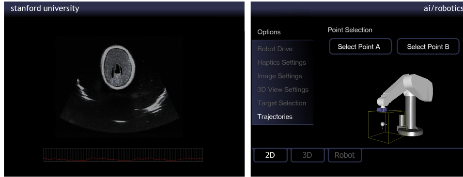
Fig. 2. Screenshot of the main interface: (Left) Visualization screen displaying a live 2D ultrasound image. (Right) Command screen which combines all operating modes and user settings of the application.
