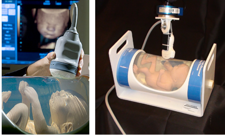
Fig. 9. (left) Illustration of the CIRS Model 068 Fetal Ultrasound Biometrics. (Right) View of the robot force sensor, transducer and fetal ultrasound phantom.
