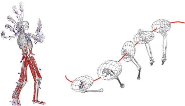
Fig. 3. Task-based analysis of muscular effort. The muscle effort variation for selected 5 configurations during a throwing motion represented by ellipsoid expansion model. The throwing hand trajectory follows the direction of the ellipsoid associated with the minimum effort [6].
