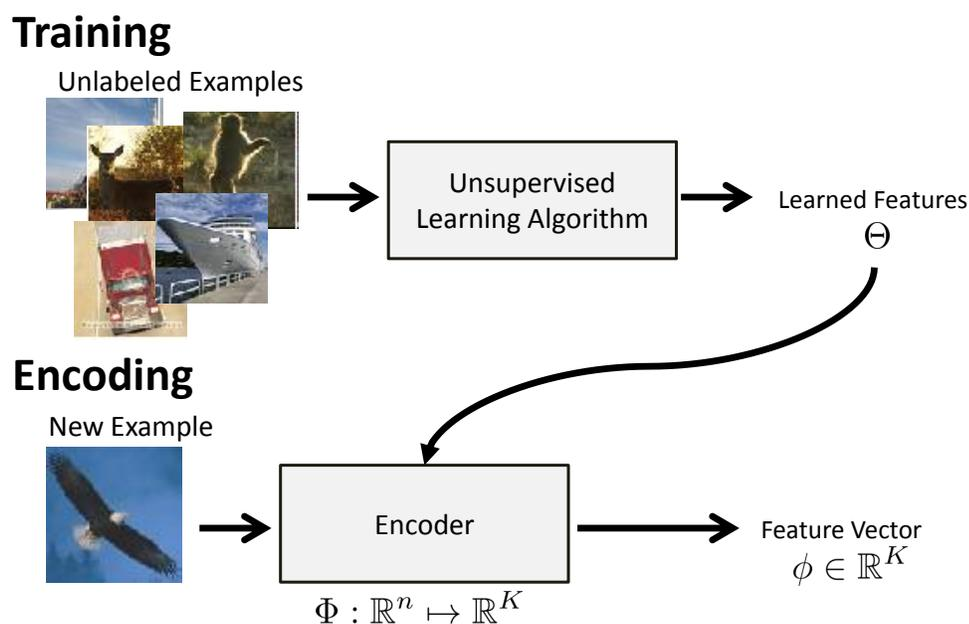
Figure 2.2: A standard template that encompasses a wide range of unsupervised feature learning algorithms.
