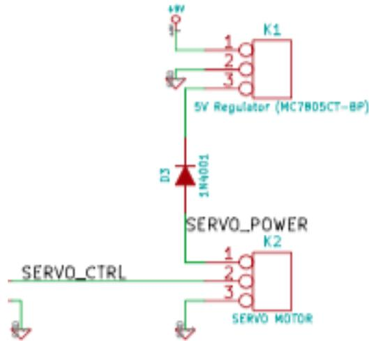
The servo motor is responsible for physically opening and closing the dog bowl. It is powered by a 9V battery that is regulated down to 5V. The servo motor uses a separate power supply due to the large amounts of current that it draws. It was also necessary to place a reverse-biased diode between the power lines of the servo motor to prevent noise from appearing on other parts of the circuit.
