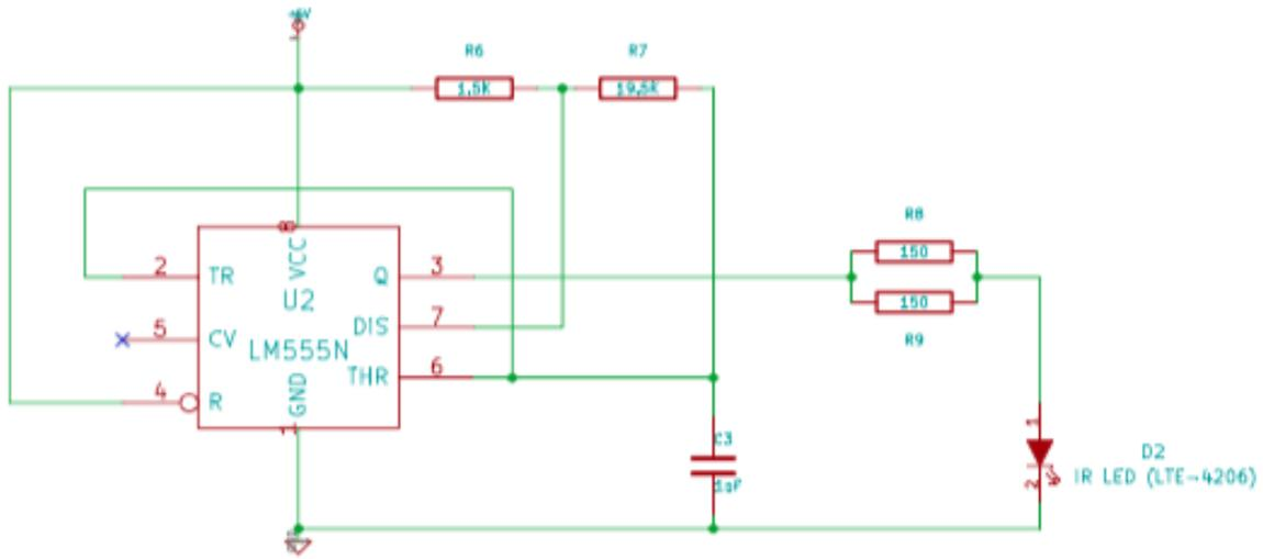
The dog tag simply uses an LM555 timer to generate a square wave. The frequency of the square wave is given by
