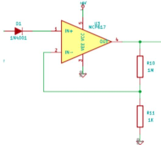
The second gain stage is nearly identical to the first. The main difference is that it receives a pure sinusoid from the bandpass filter. However, the op-amps are single supply. In order to fix this problem, a half-wave rectifier is used to block the negative portion of the sinusoid. The rectified signal is then amplified by the non-inverting gain block, which is configured to have a gain of 1000.
