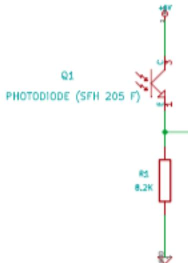
To receive the signal from the dog tag, the dog bowl has 4 photodiodes around its perimeter. These photodiodes generate current when there is incident IR light. This current is turned into a voltage by the  $8.2k\Omega$  pull-down resistor. This is how the square wave is received by the dog bowl.
