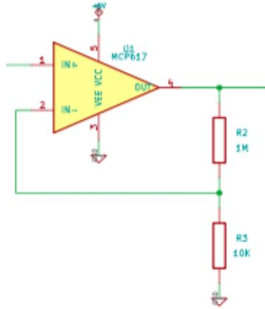
This is a simple non-inverting op-amp gain stage. The op-amp's high input impedance made this circuit a very convenient choice as a gain block. The gain of this circuit is given by
