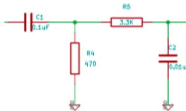
This is simply an RC highpass filter and an RC lowpass filter cascaded together. The transfer function of this arrangement is given by
