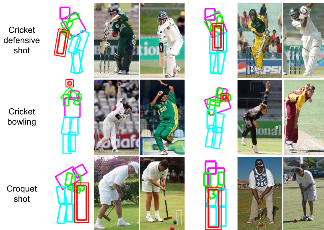
Figure 5.4: Visualization of the learned HOI models. Each row shows two models and their corresponding image examples for one activity. The illustrative figure for each model represents the average spatial layout of the object and body parts of all the images that are assigned to the model. The different color codes are: object = double red box, head and torso = magenta, arms = green, legs = cyan.)
