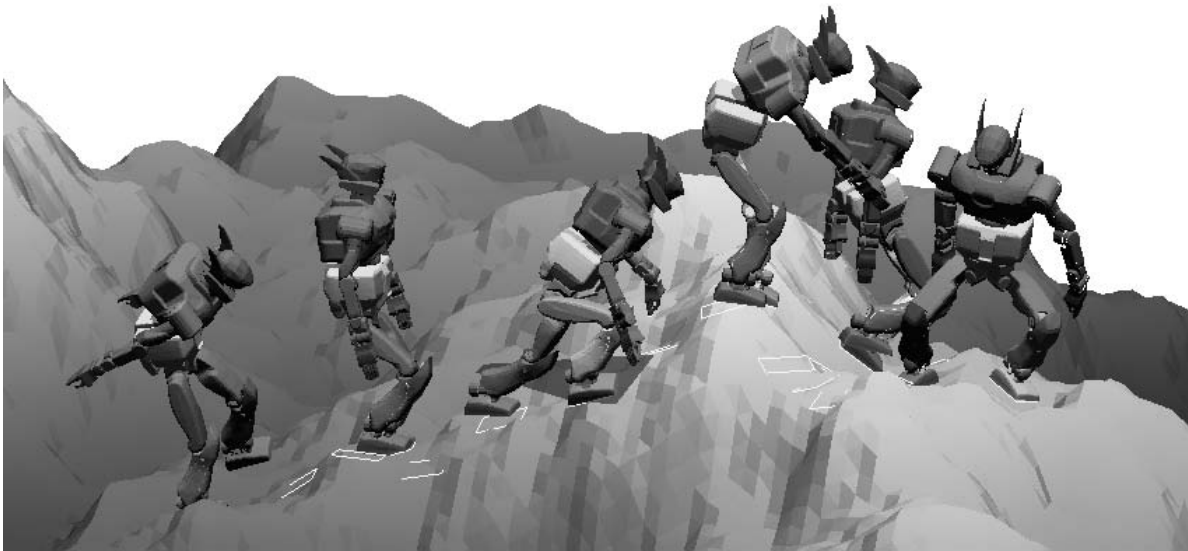
Figure 20: A motion on steep and uneven terrain generated from a set of several primitives. A hand is being used for support in the third configuration.
