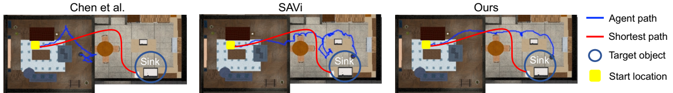
Fig. 5: Navigation trajectories on top-down maps for semantic audio-visual navigation. Chen et al. [16]: The agent gets lost near the entrance of the dining room after the sound stops. SAVi [20]: The agent struggles to avoid the obstacles and takes a long path to reach the goal. Ours: The agent successfully avoids all obstacles and efficiently navigates to the target object.
