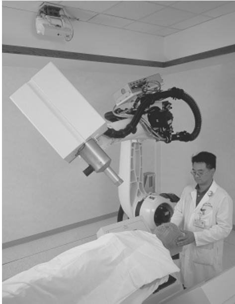
Figure 4. Photograph of the CyberKnife radiosurgery system showing: (1) ceiling mounted diagnostic X-ray sources, (2) compact linear accelerator mounted on computer-controlled robot arm, and (3) amorphous silicon detectors.
