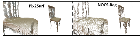
Fig. 7. Our results (left) compared with surface-agnostic X-NOCS (right), visualized with image connectivity. Pix2Surf produces significantly smoother results.
